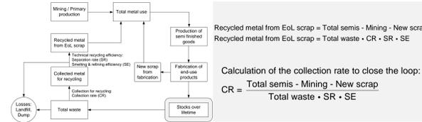
**Figure 3** Simplified methodology to enable a closed mass balance by calculating the EoL Collection Rate as a function of production data. By applying this method, the conservation of mass is enabled at every time step and the consistency of the simulated data is guaranteed.
