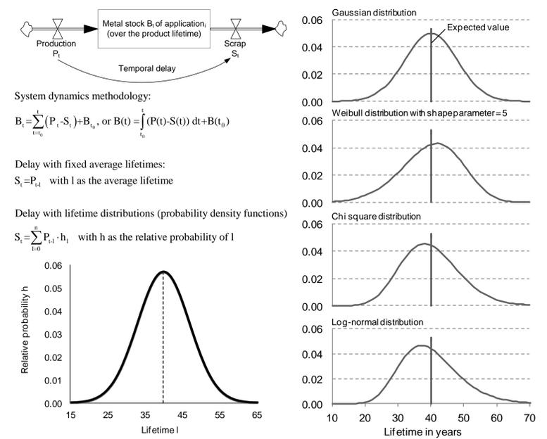
**Figure 4** Basic methodology to estimate metal stocks in use and waste flows by using different forms of temporal delays
