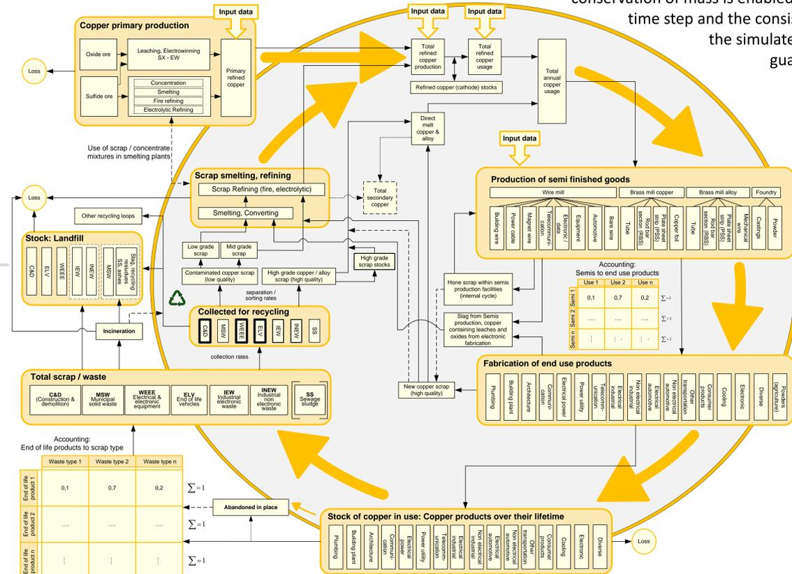
**Figure 1:** Structure of the global copper flow model
